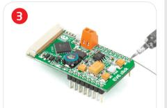
Turn the board upward again. Make sure to align the headers so that they are perpendicular to the board, then solder the pins carefully.
