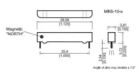
\* MK6-10-E is a magnetic latching sensor which is opened or closed by a passing magnet and remains in that state until a magnet of opposite polarity or direction passes by again. The E refers to a latching sensor and does not represent the magnetic sensitivity.
