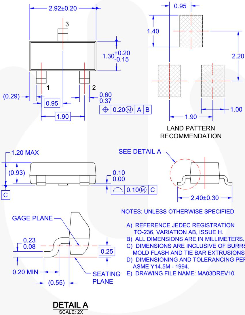
Figure 15. 3-LEAD, SOT23, JEDEC TO-236, LOW PROFILE (ACTIVE)
