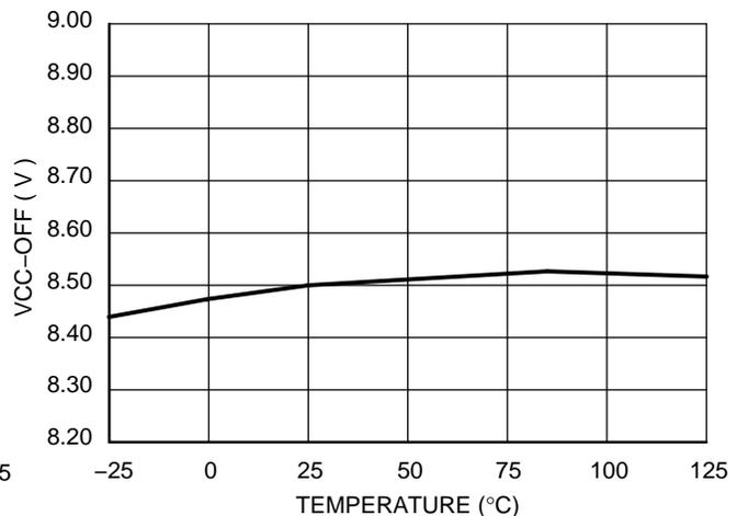
Figure 6.  $V_{CC}$  OFF, FB = 1.5 V vs. Temperature
