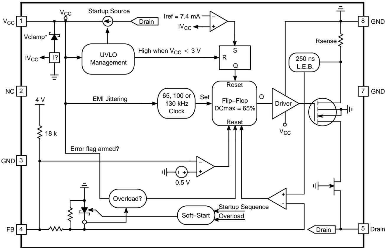
\*V<sub>clamp</sub> = V<sub>CCOFF</sub> + 200 mV (8.7 V Typical)
