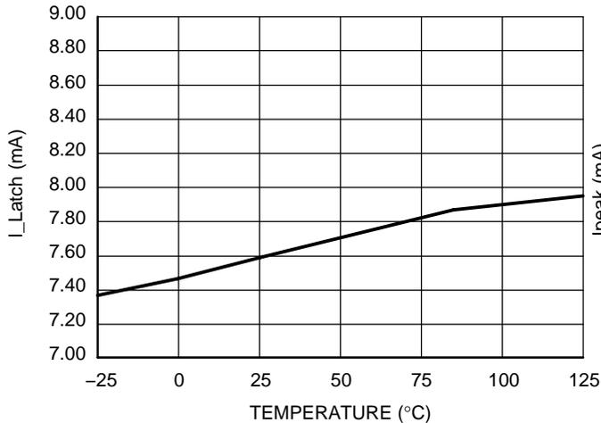
Figure 9. I<sub>Latch</sub>, FB = 1.5 V vs. Temperature
