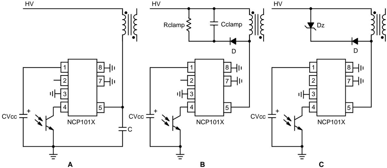
**Figure 27. Different Options to Clamp the Leakage Spike**
