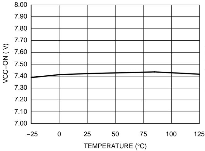
Figure 7. V<sub>CC ON</sub>, FB = 3.5 V vs. Temperature
