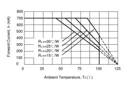
Note: Don't drive at rated current more than 5s without heat sink for Xeon 3 emitter series.
