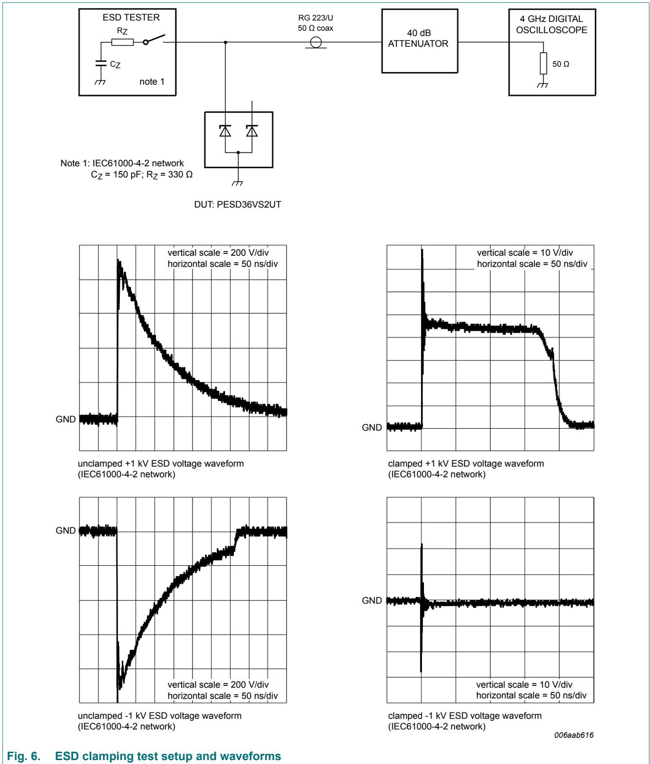
Fig. 6. ESD clamping test setup and waveforms
