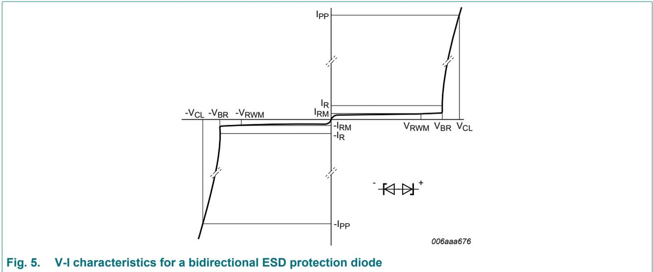
Fig. 5. V-I characteristics for a bidirectional ESD protection diode
