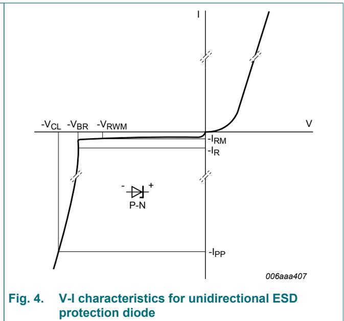
Low capacitance unidirectional double ESD protection diode
