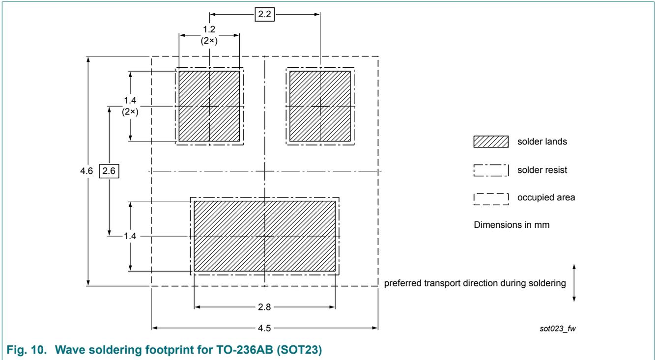
Fig. 10. Wave soldering footprint for TO-236AB (SOT23)
