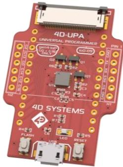
This connects to the pixxiLCD display through a 15-way-to-30-way cable.
