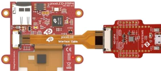
The 4D-UPA is used to update the PmmC and to download compiled 4DGL code into the processor. It also serves as an interface for communicating serial data to the PC.
