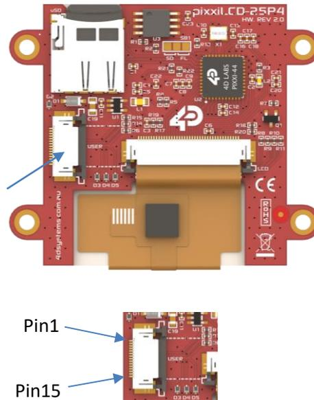
Figure 2: FPC Pinout
