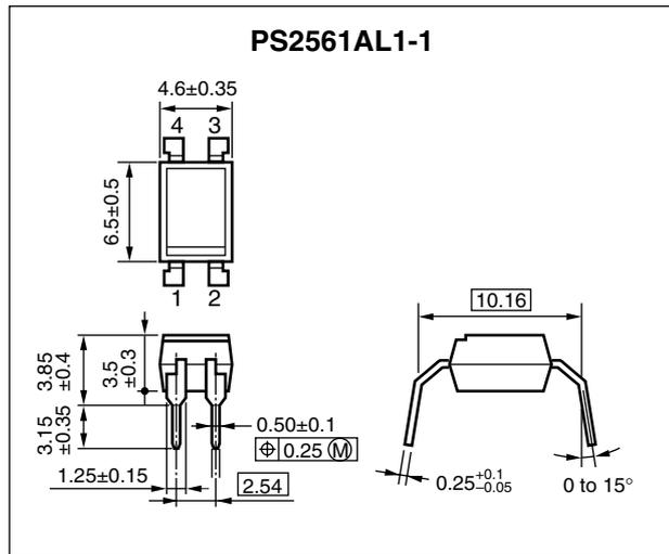
Lead Bending Type (Gull-Wing)
