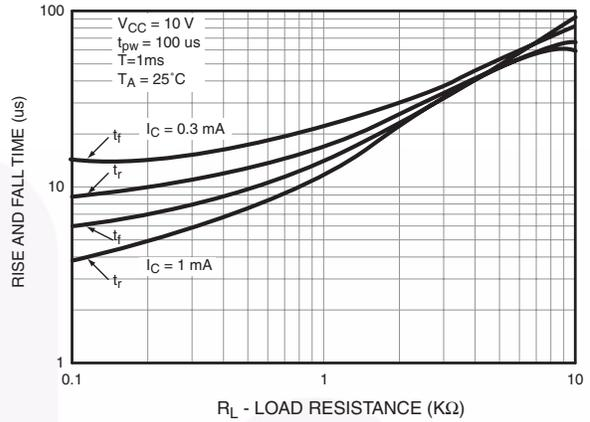
Fig. 7 Rise and Fall Time vs. Load Resistance
