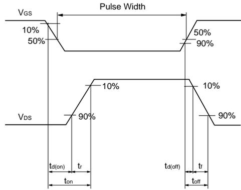
Fig.11 Switching Waveforms
