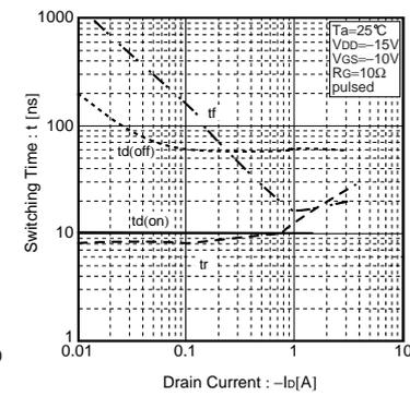
Fig.8 Switching Characteristics
