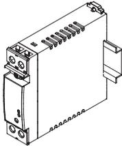
Horizontal mounting with DIN rail
