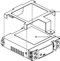
\*Mounting with DIN rail is not possible when mounting facing horizontally.
