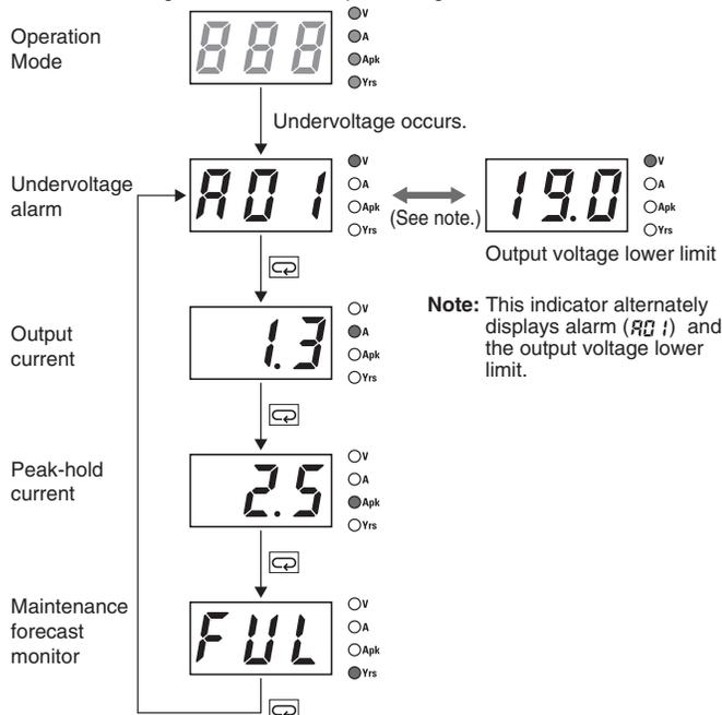
**Note:** 1. The display changes to the output voltage display when the voltage is restored to the set value or higher.
