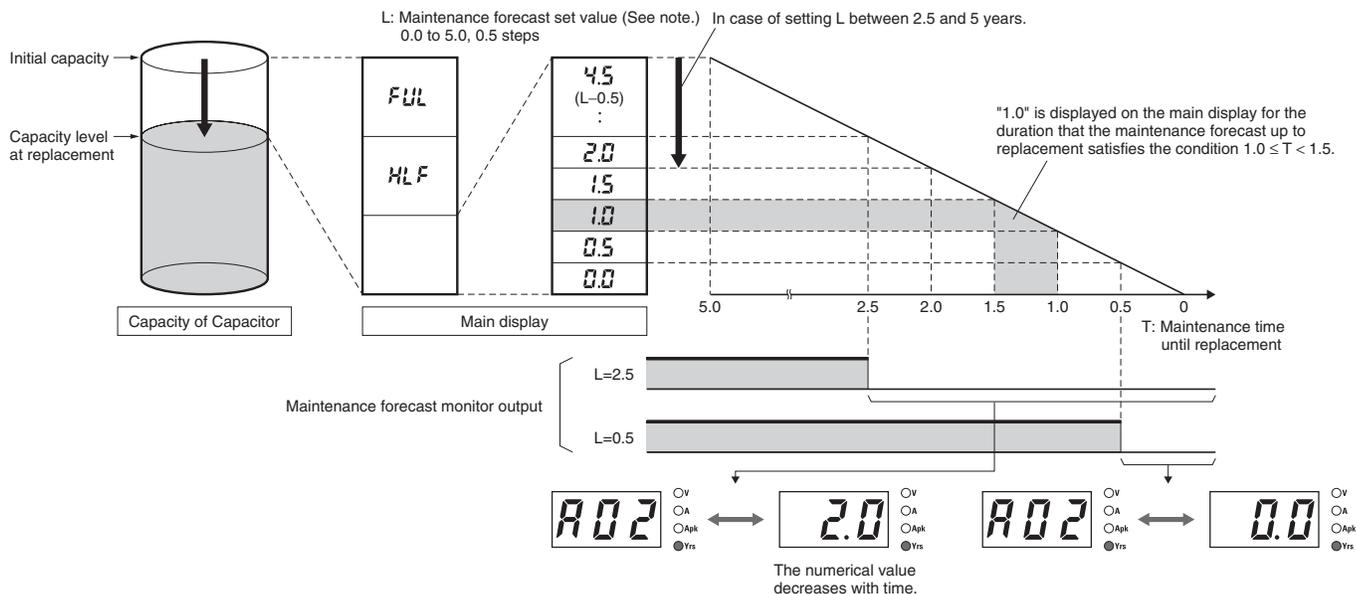
**Note:** This function can be set only on the S8VS-09024A□, S8VS-12024A□, S8VS-18024A□, and S8VS-24024A□.
