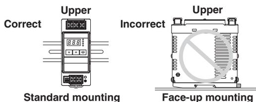
**Note:** Improper mounting will interfere with heat dissipation and may occasionally result in deterioration or damage of internal parts. It may also result in failure of the maintenance forecast monitor function. Use the standard mounting method only.
