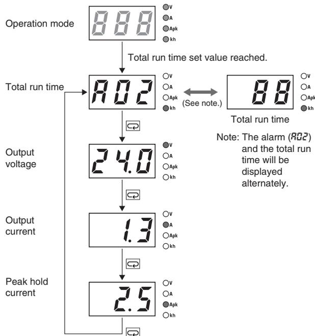
The accumulated value of the operating time of the Power Supply is displayed as the total run time. 0 (kh) will be displayed initially after purchase and then the display will advance in 1-kh steps as the operating time accumulates. When the total run time reaches the preset alarm set value, the alarm (R02) and the total run time will be displayed alternately and a transistor ((12) total run time output terminal (kh)) will output the status externally.
