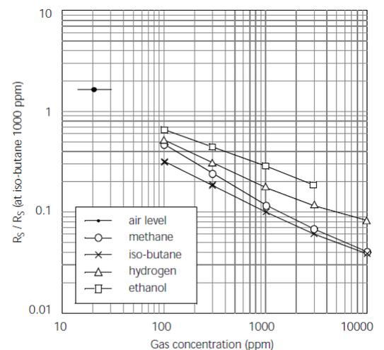
Fig3. Sensitivity characteristics
