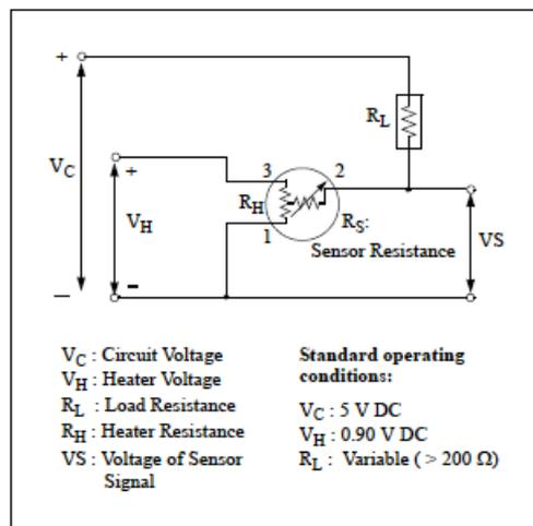
Fig 2. Standard circuit
