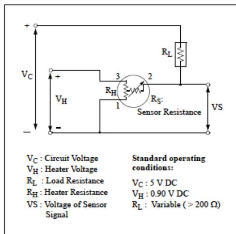
Fig 3. Standard circuit
