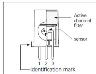
Fig 1c. Pin Layout
