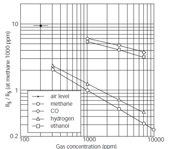
Fig4. Sensitivity characteristics
