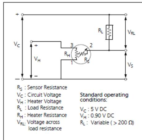
Fig 2. Standard circuit
