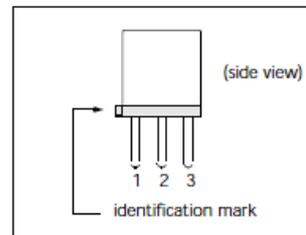
Fig 1c. Pin Layout
