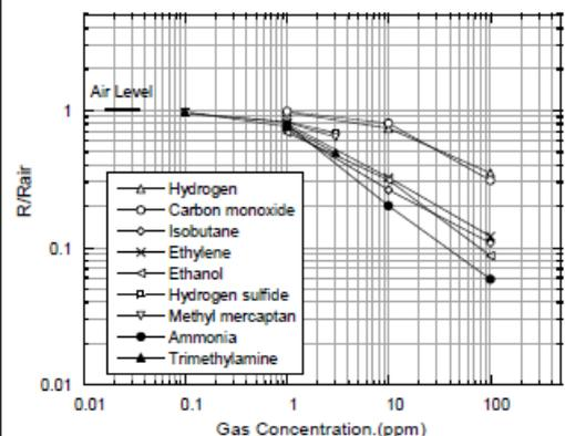
Fig 3. Sensitivity characteristics
