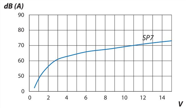
All measurements are made @ 12Vdc @ 1 meter in free air @ 21°C.
