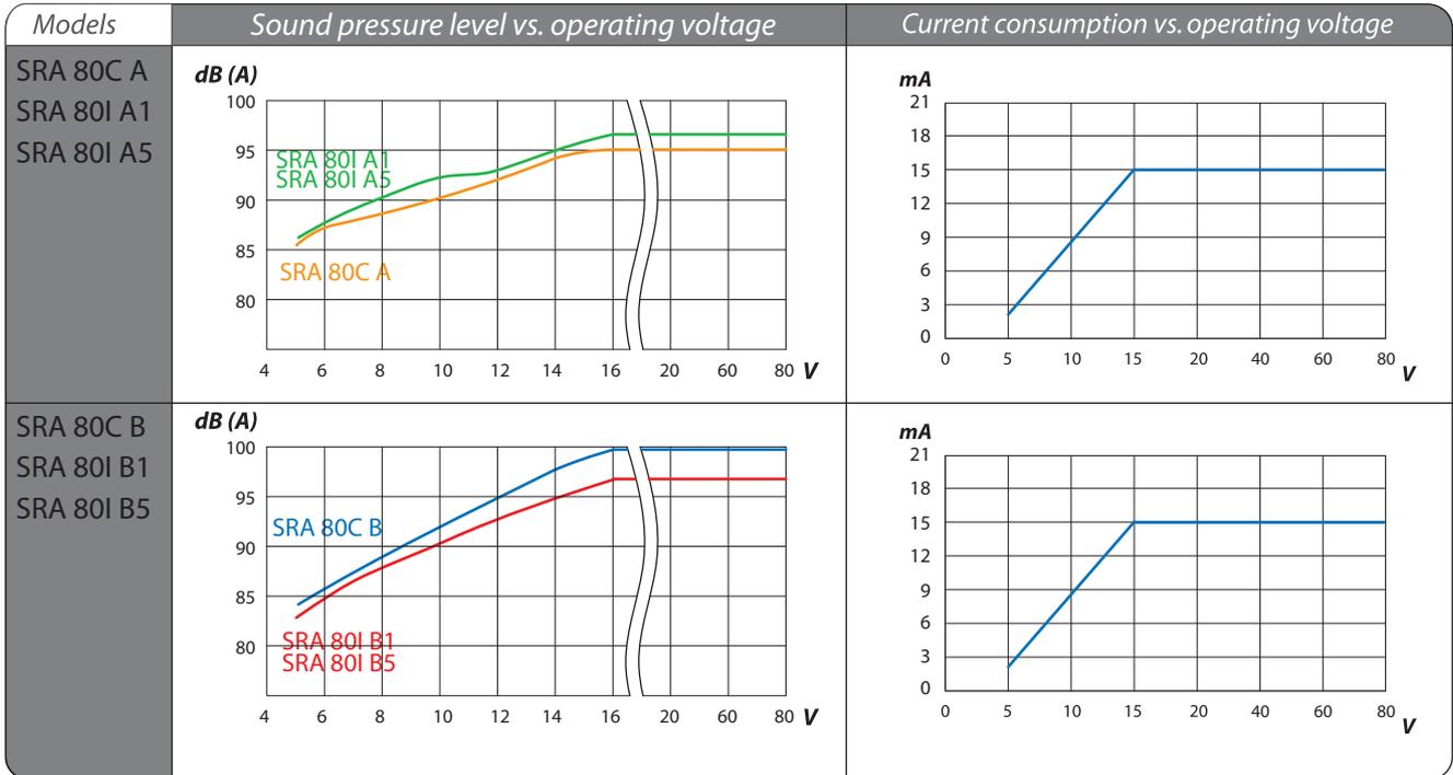
All measurements are made @ 12Vdc @ 1 meter in free air @ 21°C.
