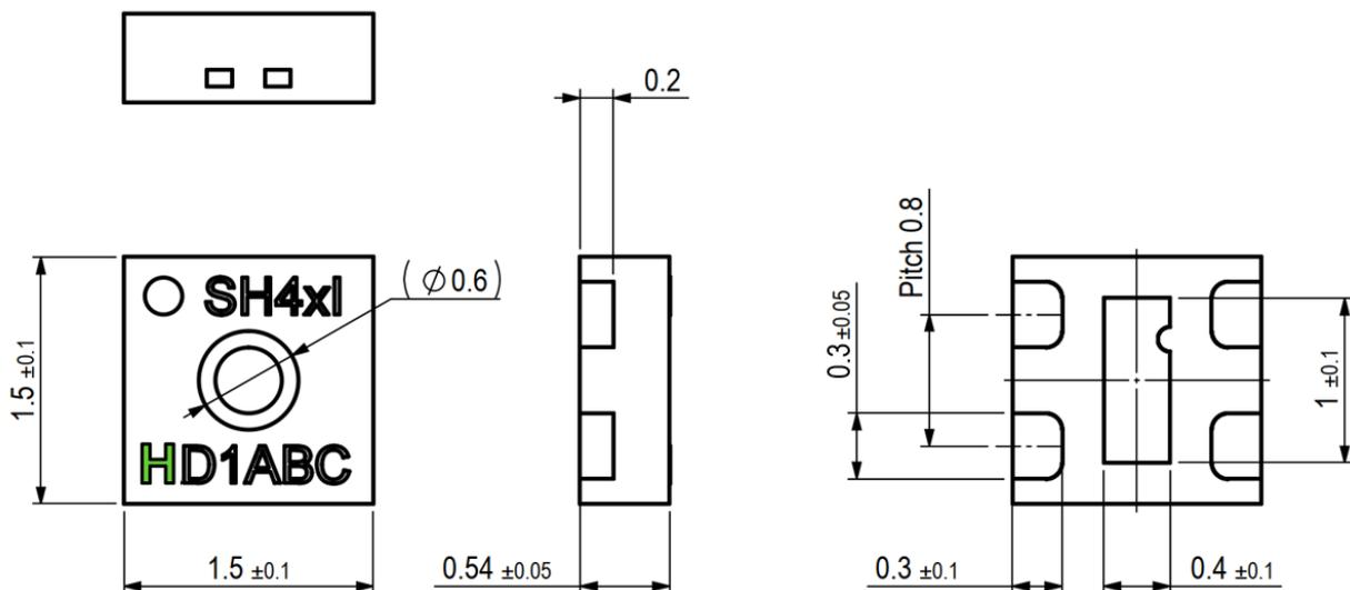
**Figure 8:** Dimensional drawing of SHT40I analog including package tolerances (units mm), where the H (here highlighted in green for better identification) serves as indicator for the standard analog interface. Other letters alphabetically after the letter H, indicate other versions of the analog interface, as detailed in **Table 11** and described in section 4.4.
