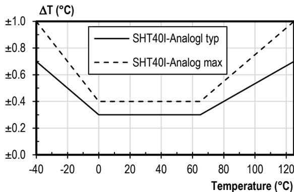
**Figure 2:** SHT40I analog (output characteristics H,I,J, K, *vide infra*) typical and maximal temperature accuracy, where model SHT40I-ID1B is only specified between -20°C and +80°C.
