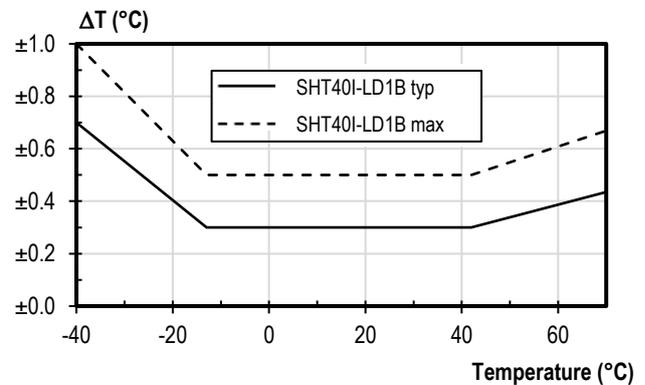
**Figure 3:** SHT40I-LD1B typical and maximal temperature accuracy.
