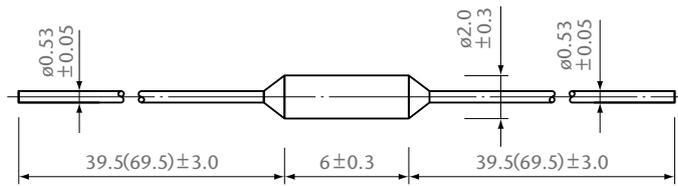
Note: The dimensions for long lead devices are in parentheses.
