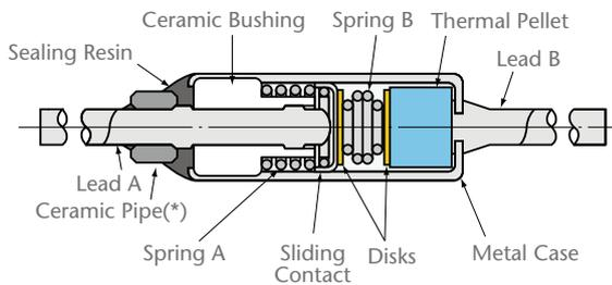
The SF-type contains a sliding contact, springs and a thermal pellet inside a metal case. When spring B is compressed, there is firm contact between lead A and the sliding contact. At normal temperatures, current flows from lead A to the sliding contact and then through the metal case to lead B.
