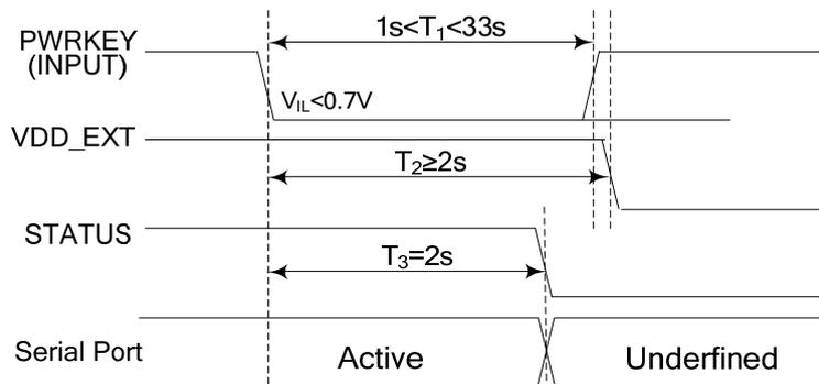
**Figure 13: Timing of power off SIM800F by PWRKEY**
