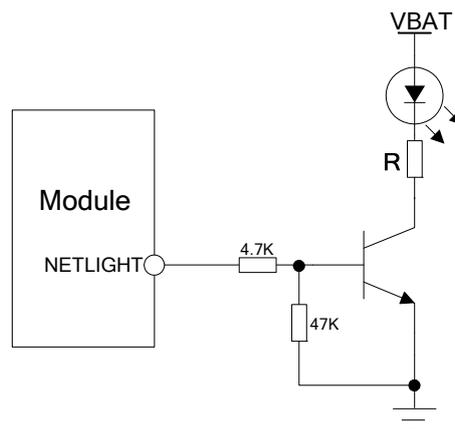
**Figure 39: Reference circuit of NETLIGHT**
