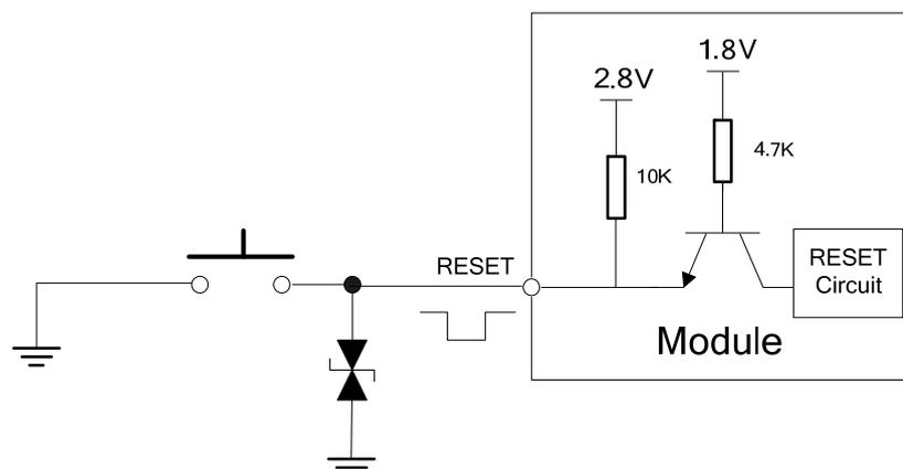
Figure 15: Reset Circuit
