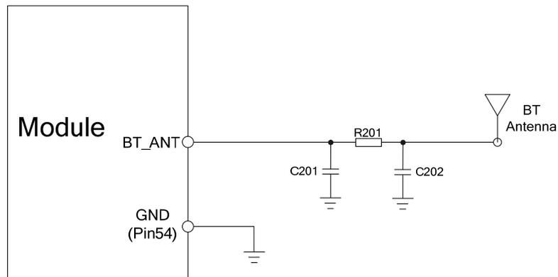
**Figure 44: Bluetooth antenna matching circuit**
