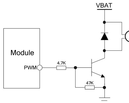
**Figure 40: Reference circuit of PWM drive buzzer**
