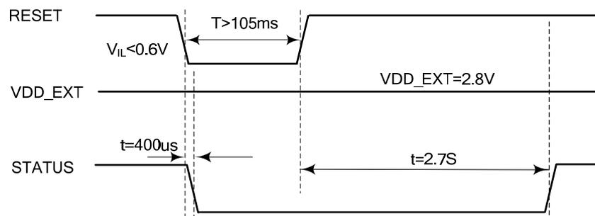
**Figure 16: Reset timing**
