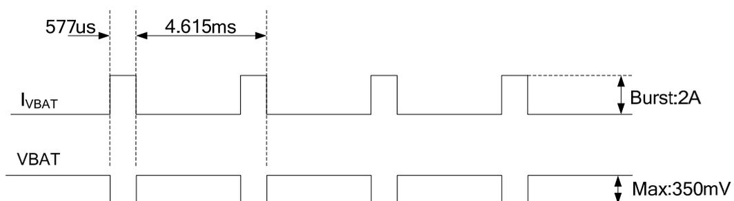
**Figure 8: VBAT voltage drop during max power transmitting**
