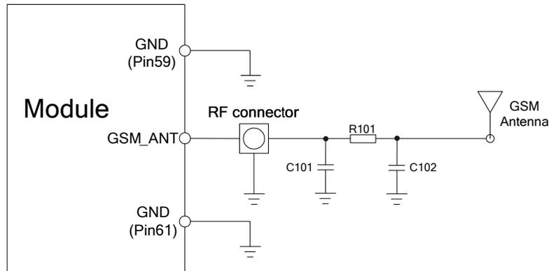
**Figure 42: GSM antenna matching circuit**
