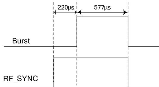
**Figure 38: RF\_SYNC signal during transmit burst**
