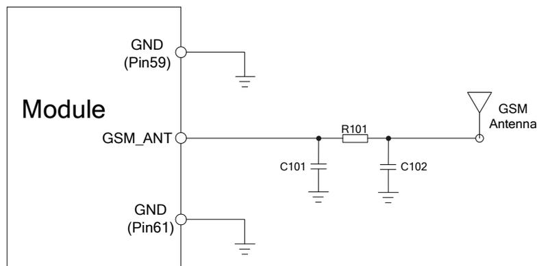
**Figure 43: GSM antenna matching circuit without RF connector**
