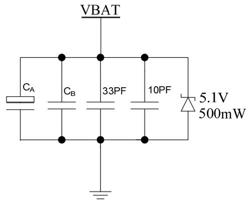
**Figure 7: Reference circuit of the VBAT input**
