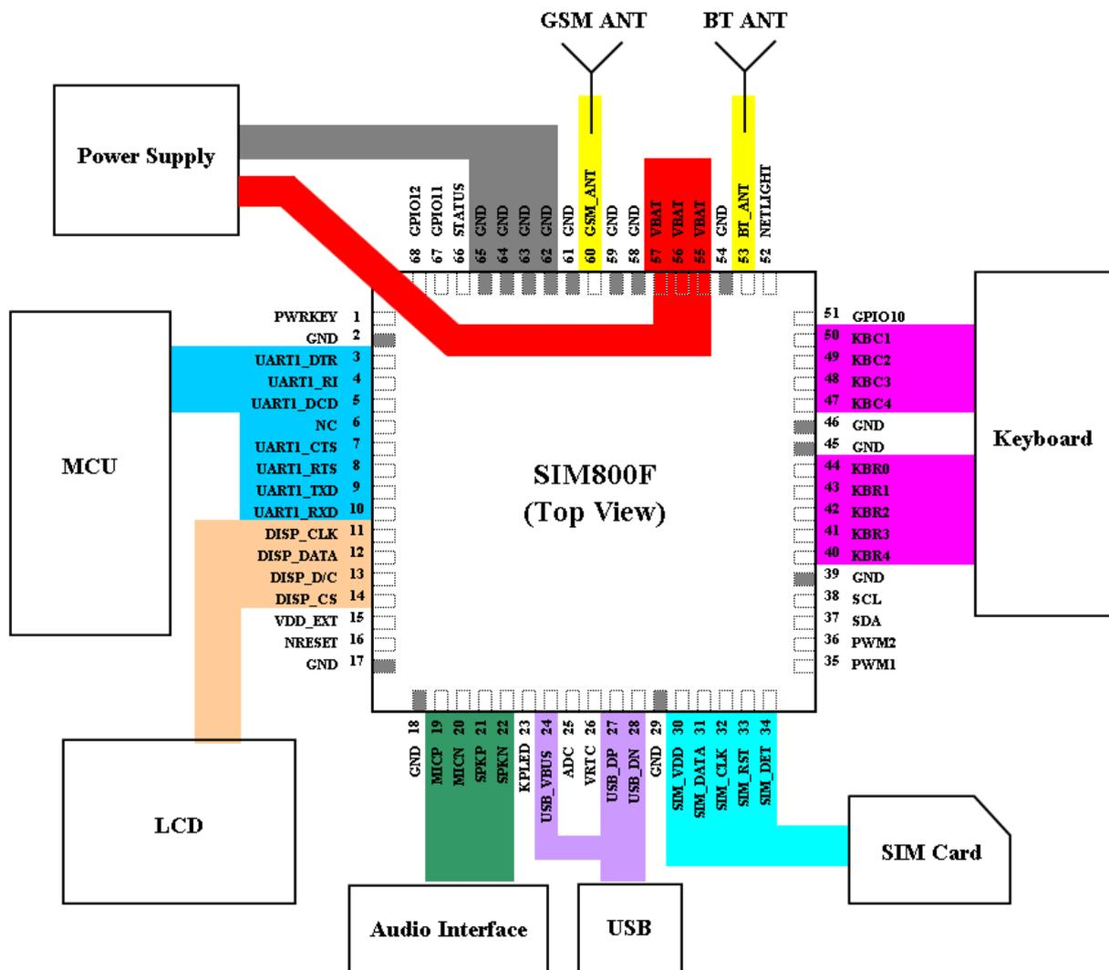
Figure 45: Pin assignment
