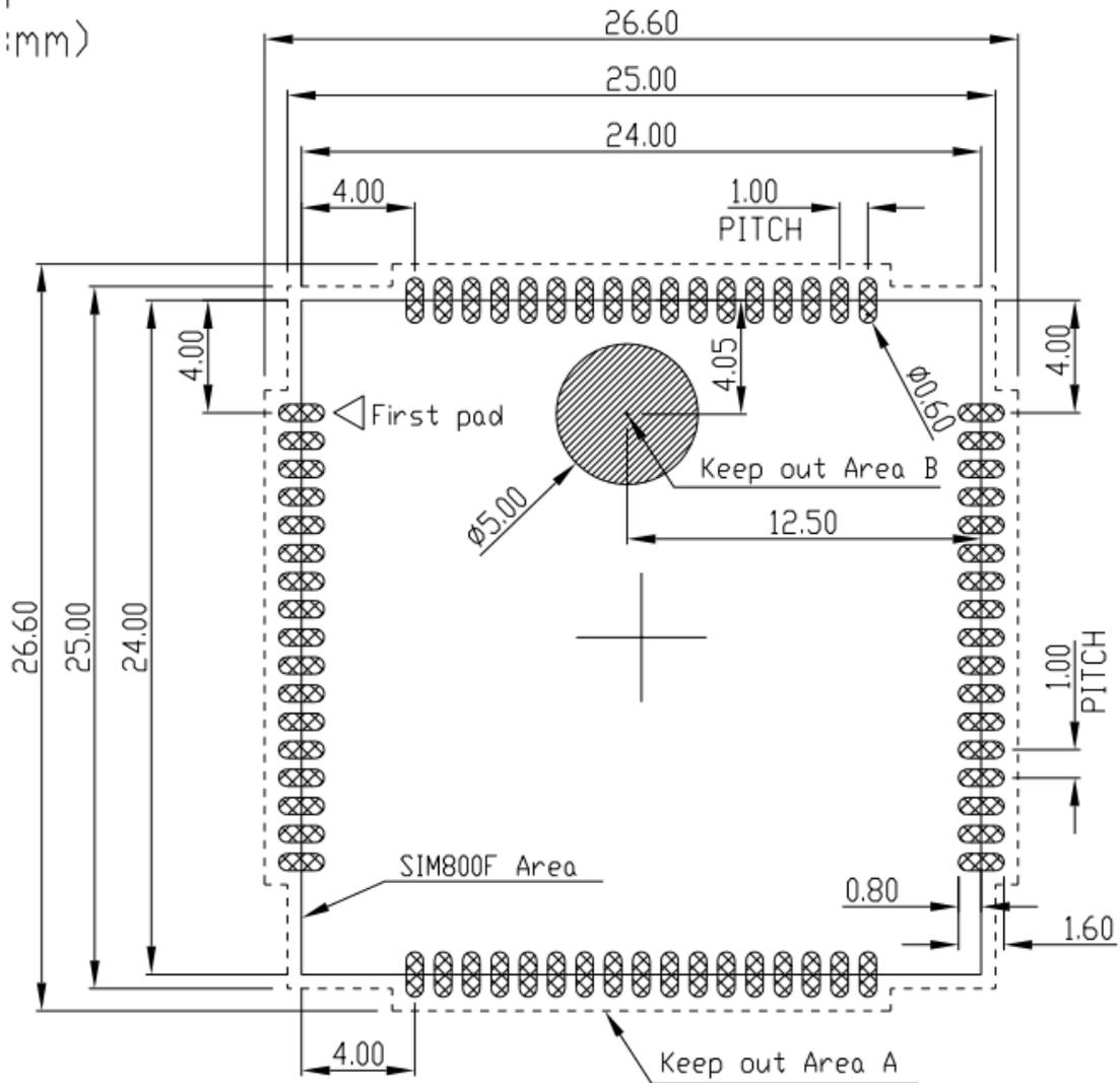
**Figure 4: Recommended PCB footprint outline (Unit: mm)**
