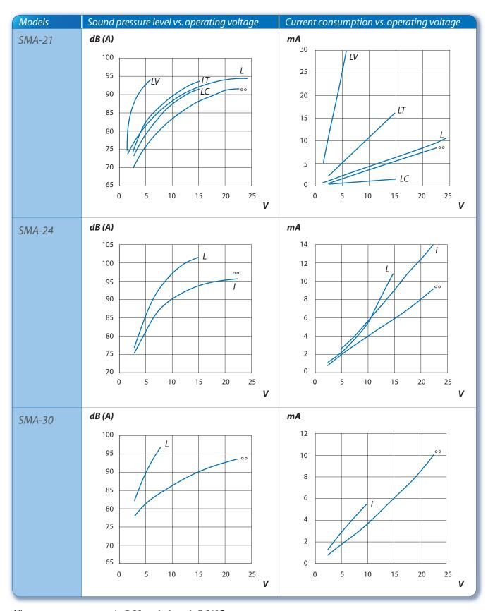
All measurements are made @ 30 cm in free air @ 21°C. °°: standard versions, respectively SMA-21, SMA-24, SMA-30.
