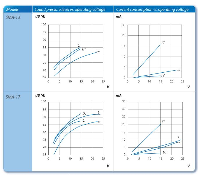
All measurements are made @ 30 cm in free air @ 21°C. °°: standard versions, respectively SMA-13, SMA-17.
