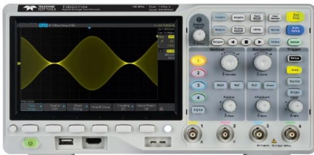
Front panel of T3DSO1104, T3DSO1202A, T3DSO1204, T3DSO1302A
