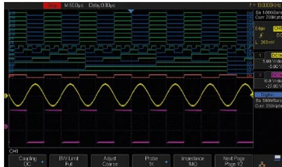
16 digital channels enables users to acquire and trigger on the waveforms then analyze the pattern, simultaneously with one instrument. Color coded logic levels clearly differentiate high and low states.
