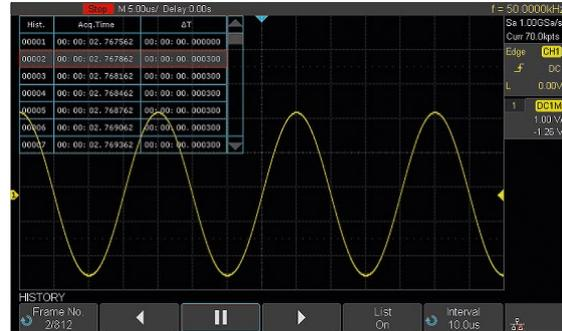
Playback the latest triggered events using the history function. Segmented memory collection will store trigger events into multiple (Up to 80,000) memory segments, each segment will store triggered waveforms and timestamp each frame.
