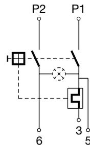
2 pole thermal overload protection
