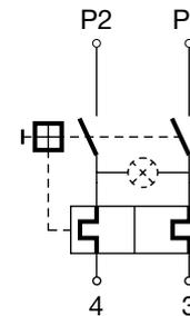
2 pole thermal overload protection, Shunt terminal
