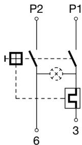
1 pole thermal overload protection, Shunt terminal
