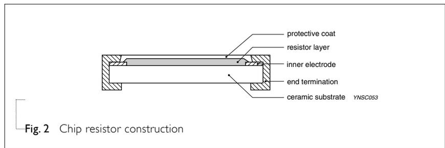
Fig. 2 Chip resistor construction
