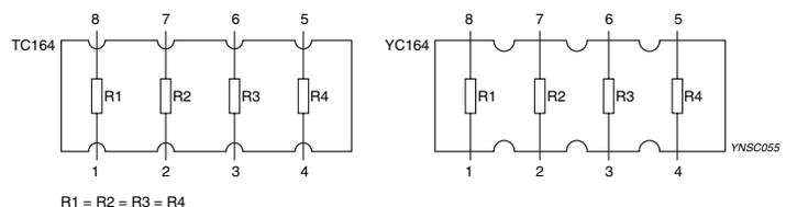
Fig. 4 Equivalent circuit diagram
