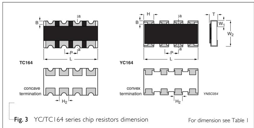
Fig. 3 YC/TC164 series chip resistors dimension
