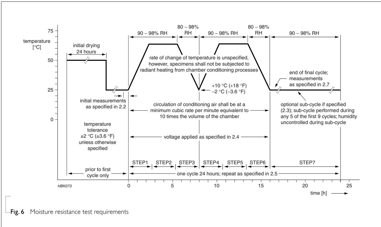
Fig. 6 Moisture resistance test requirements
