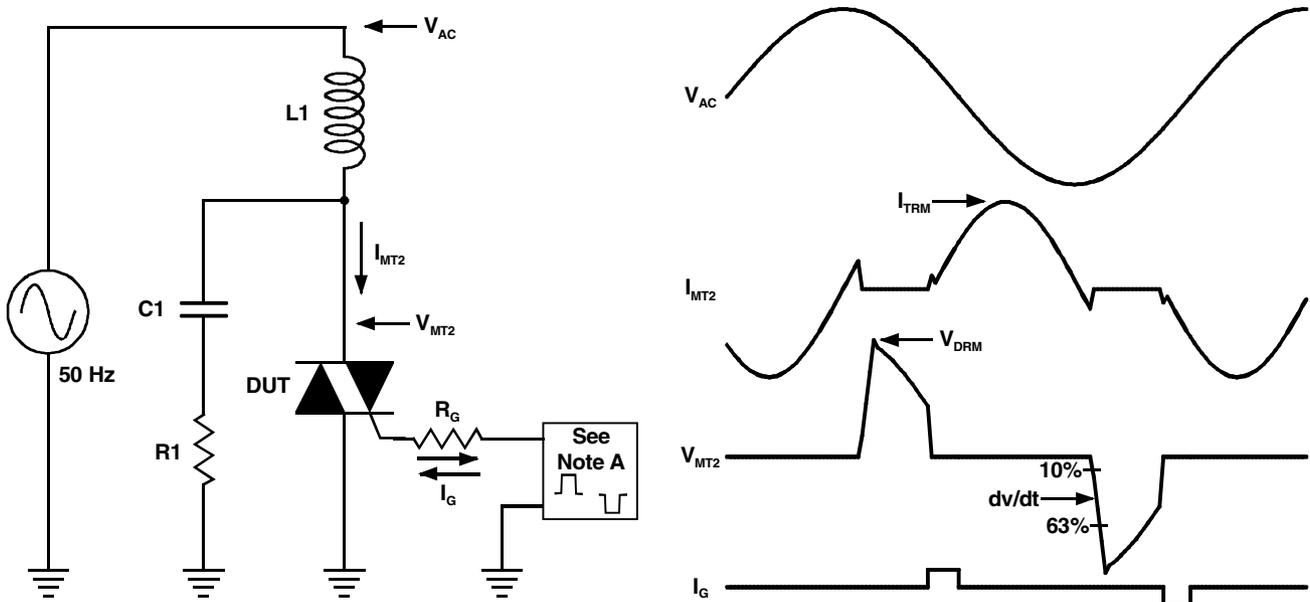
NOTE A: The gate-current pulse is furnished by a trigger circuit which presents essentially an open circuit between pulses. The pulse is timed so that the off-state-voltage duration is approximately 800  $\mu$ s.
