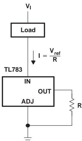
Figure 21. Current-Sinking Regulator
