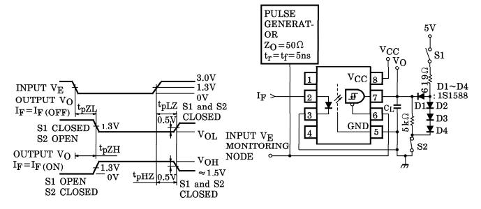
C<sub>L</sub> is approximately 15pF which includes probe and stray wiring capacitance.
