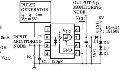
$C_1$  is peaking capacitor. The probe and jig capacitances are include in  $C_1$ .
