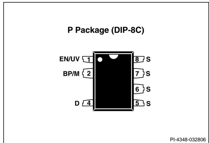
Figure 3. Pin Configuration.
