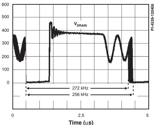
Figure 4. Frequency Jitter.
