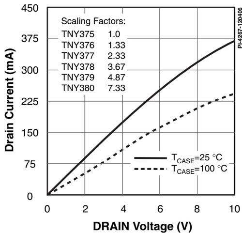
Figure 25. Output Characteristics.
