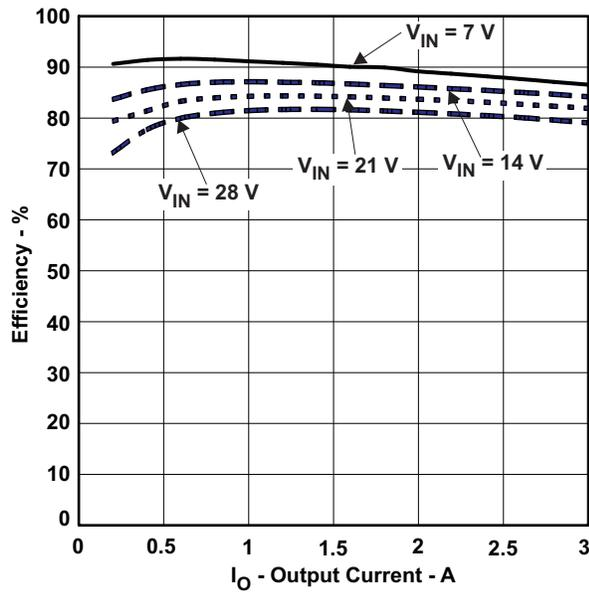
Figure 15. TPS54331 Efficiency
