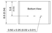
Dimensions in mm (inch) Tolerances: x.xx  $\pm 0.5$  ( $\pm 0.02$ ) Tolerances: x.xxx  $\pm 0.25$  ( $\pm 0.01$ ) Pin dimension tolerances:  $\pm 0.10$  ( $\pm 0.04$ )
