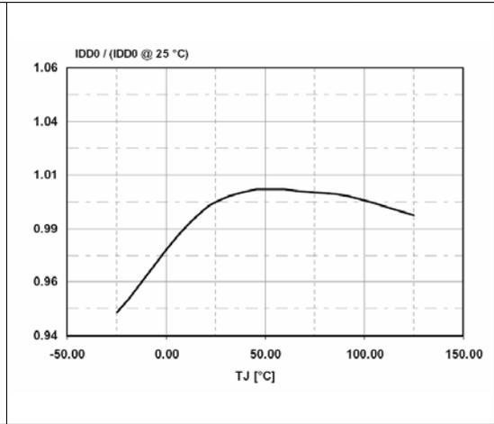
Figure 15. Operating supply current (switching) vs  $T_J$
