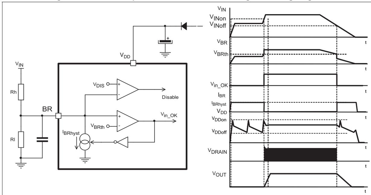
Fixed the  $V_{INon}$  and the  $V_{INoff}$  levels, with reference to [Figure 31](#), the following relationships can be established for the calculation of the resistors  $R_H$  and  $R_L$ :
