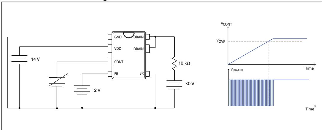
Note: Adjust V<sub>DD</sub> above V<sub>DDon</sub> start-up threshold before settings to 14 V
