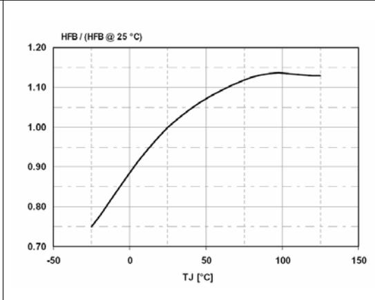
Figure 11. Brown out threshold vs  $T_J$
