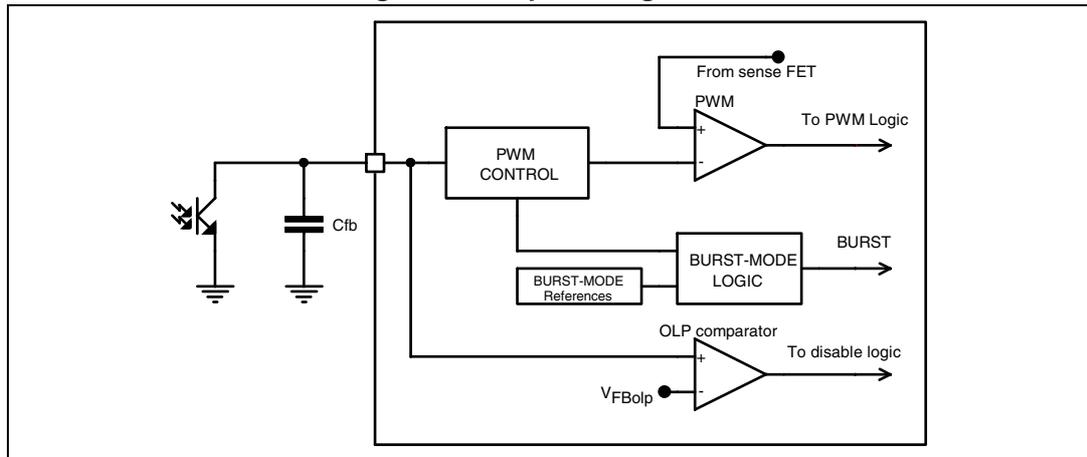
Figure 29. FB pin configuration
