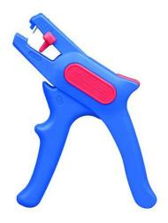
The WEICON Wire Stripper No. 5 has an adjustable length stop from 5 - 12 mm. This allows all flexible and solid conductors of 0.2 - 6.0 mm² (24 - 10 AWG) to be stripped. The length stop can be removed if required. An easy-to-access side cutter is integrated into the tool and can be used up to a cable diameter of 2 mm. It also has exchangeable blades.
