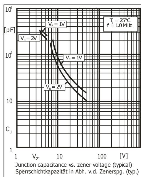
Junction capacitance vs. zener voltage (typical)
