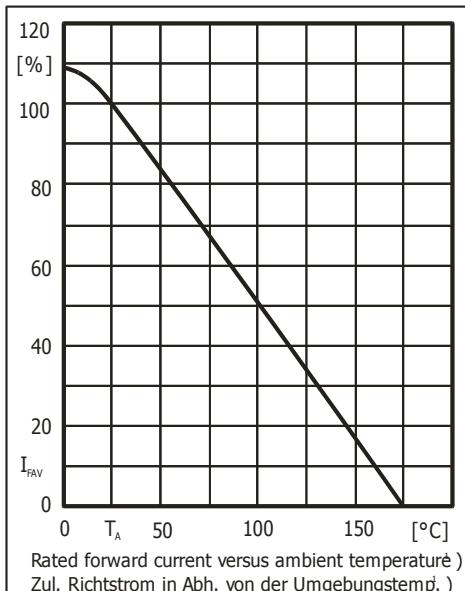
Rated forward current versus ambient temperature )
